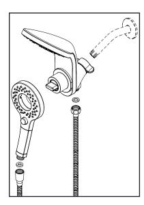
(1) Apply Teflon tape on the threaded end of shower arm, hand tighten inlet end of handheld shower holder to shower arm threaded end then tighten and align handheld shower holder with help of adjustable wrench. With washer inside the hose connection nut hand tighten hose connection nut to outlet end of handheld shower holder then tighten hose connection nut with help of adjustable wrench.
