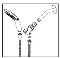
(1) Apply Teflon tape on the threaded end of shower arm, hand tighten inlet end of handheld shower holder to shower arm threaded end then tighten and align handheld shower holder with help of adjustable wrench. With washer inside the hose connection nut hand tighten hose connection nut to outlet end of handheld shower holder then tighten hose connection nut with help of adjustable wrench.
