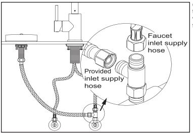
(8) Attach and tighten both 3/8" end of inlet supply hoses to tee with help of adjustable wrench. Turn on angle stop valves to check for leaks and make sure glass washer functions properly.
