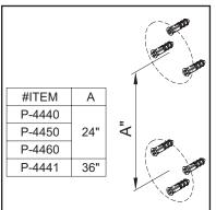
(1) Locate where to install the slide/grab bar and use a pen to mark the location of all six mounting screws. Use a power drill to drill 5/16" screw holes. Insert the screw anchors into the holes and hammer them flush to the wall as shown in the drawing.
