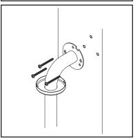
(2) Secure the slide/grab bar on the wall by tightening the mounting screws into the screw anchors. Place both flanges to cover the mounting screws as shown in the drawing.
