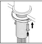
(4) Thread locknut onto the faucet shank from underneath the sink. Position faucet to desired location from the top and hand-tighten locknut till it won't go further. Thread both screws on locknut and tighten screws on locknut with the help of a Phillips head screwdriver to secure faucet. (Note: Do not overtighten.)
