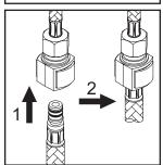
(6) Insert spray head hose into end of quick connect adapter on the outlet hose, push until a "click" is heard. Pull down to test engagement.
