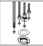
(3) With flat side of the locknut facing down and the steel washer inside the locknut please follow the order as the drawing shows to insert flex hoses through the center hole of the locknut from underneath the sink.
