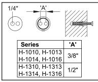
(1) Please refer the 'A' distance on the chart and locate where to install based on the model you have then use a power drill to drill two 1/4" mounting holes.
