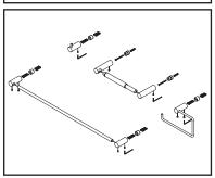
(3) Secure the bathroom hardware with the screw at the bottom. Do not overtighten.
