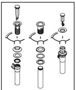
(2) a. For brass pop-up: Place a ring of plumbers putty on the bottom of the flange and apply Teflon tape on threaded tailpiece. Thread tailpiece to drain body. Insert flange through drain hole and attach drain body to flange from underneath the sink.
