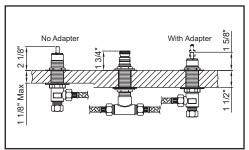
(1) Please refer to the drawing for required valve and shank height from finished surface when install the valve.
