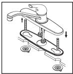
(2) Apply adequate plumbers putty along the boundary of base gasket. Thread mounting bolts to the bottom of faucet. Align faucet with mounting holes and place faucet on the sink, thread locknut onto mounting bolts from underneath the sink, hand tighten locknuts. Go to step (5) if faucet is without side spray.
