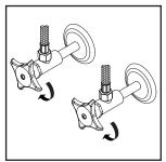
(1) Shut off the water supply. Remove old faucet. Clean mounting surface in preparation
