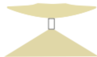
Batwing Indirect Lighting
