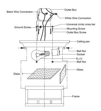
STEP 6: Install the glass panels into the frame, and then combine the fixture with the frame, and fasten it with the ball nut.
