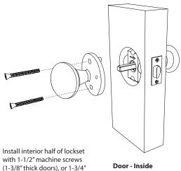
machine screws (1-3/4" thick
