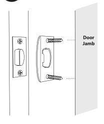
Attach the strike plate to the door jamb using 3/4" long wood screws.
