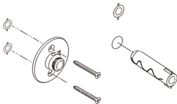
⑤ INSTALL PRODUCT ONTO BRACKETS AND TIGHTEN THE ESCUTCHEON
