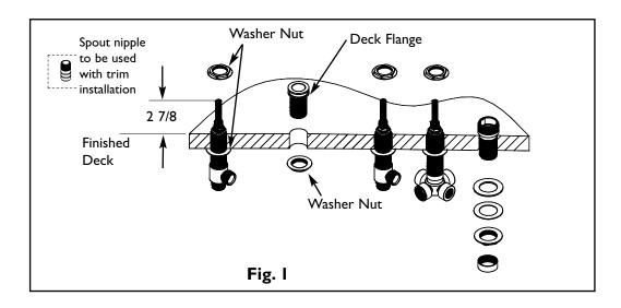
3. Attach hot/cold valves to spout, utilizing 3/4" copper pipe. See Fig. 2
