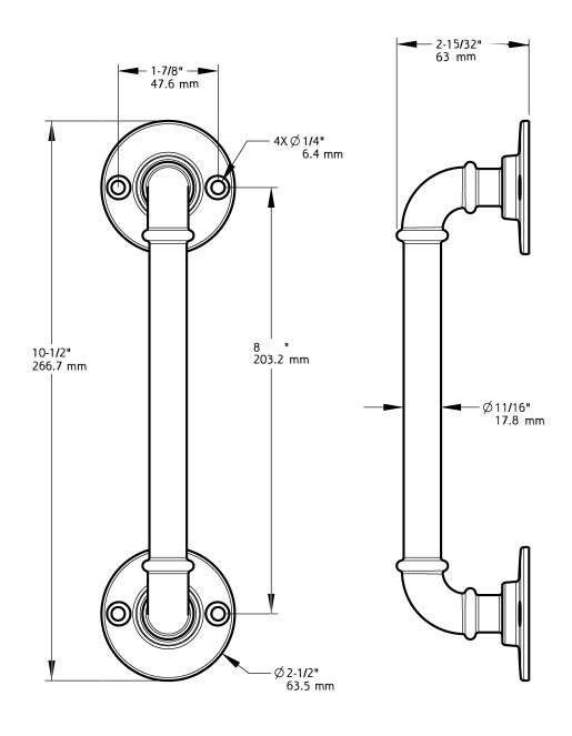
Material: Steel Fasteners: (4) #12 X 1-1/2",Type AB, Oval Head, Tapping Screw
