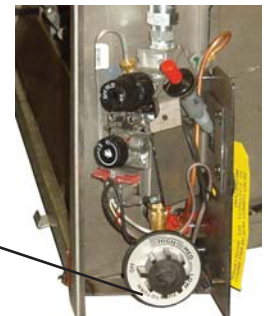
Rear burner control knob
