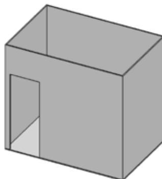
Within a partial enclosure which includes an overhead cover and no more than two sidewalls. These sidewalls may be parallel, as in a breezeway, or at right angles to each other.
