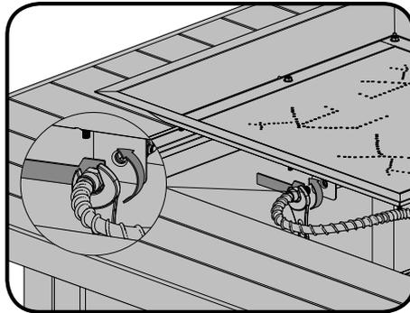
4. Unscrew the propane orifice from the inside of the burner as illustrated.
