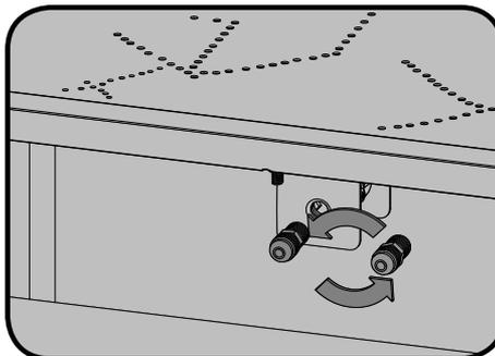
5. Replace the propane orifice with the natural gas orifice supplied.
