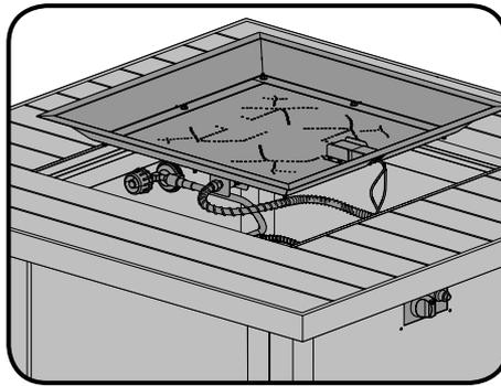
3. Disconnect the stainless steel flex connector from the orifice using (2) wrenches.
