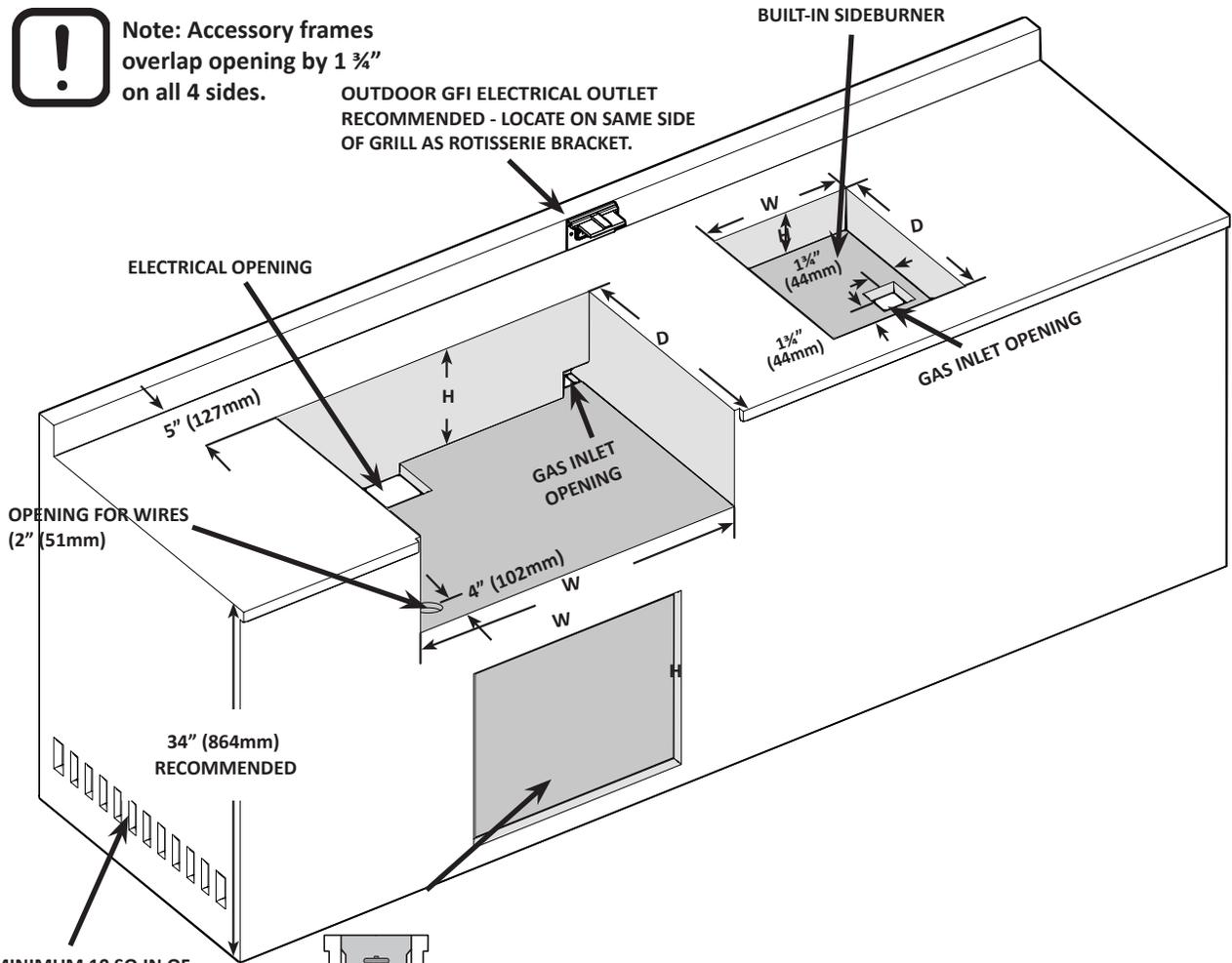
MINIMUM 10 SQ IN OF VENTILATION REQUIRED ON EACH END OF CABINET
