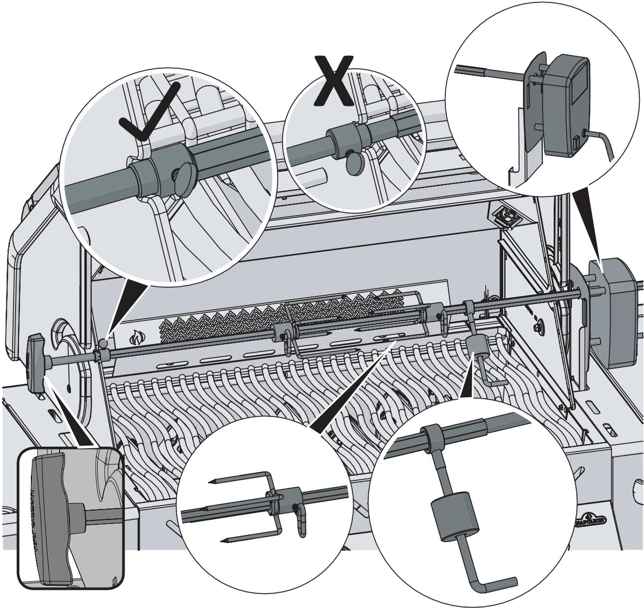
**Ensure stop bushing is tightened on the inside of hood casting.**
