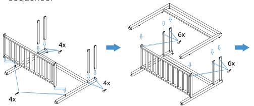
Do not tighten bolts completely!
