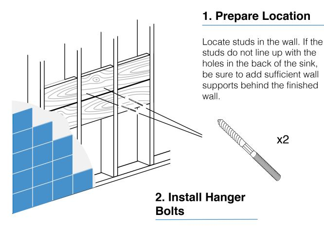
Measure the distance between mounting holes in the back of the sink. Drill pilot holes in wood and screw in hanger bolts. Check postion with a level.
