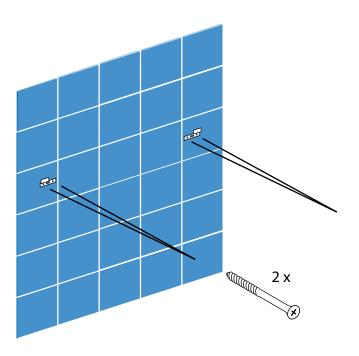
Mark the desired height of the vanity on the wall. Mark the location of the vanity. Drill pilot holes and install the mounting brackets. Check position with a level.
