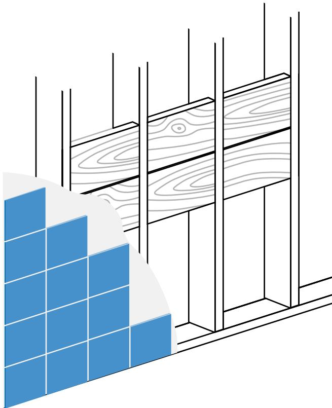
Locate studs in the wall. If the studs do not line up with the holes in the back of the sink and vanity, be sure to add sufficient wall supports behind the finished wall.
