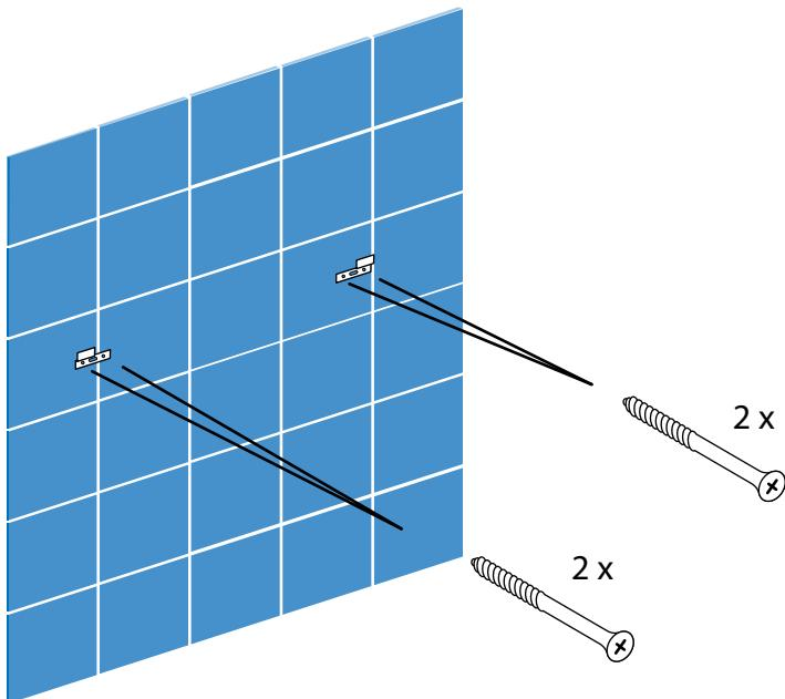
Mark the desired height of the vanity on the wall. Mark the location of the vanity. Drill pilot holes and install the mounting brackets. Check position with a level.
