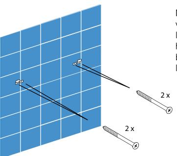
Mark the desired height of the vanity on the wall. Mark the location of the vanity. Drill pilot holes and install the mounting brackets. Check position with a level.
