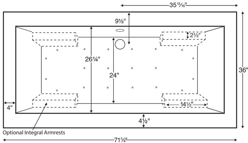
The Sculpted Finish process does not allow enough space for mounting fixtures on the tub deck.
