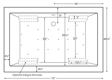
The Sculpted Finish process does not allow enough space for mounting fixtures on the tub deck. Shown as Air Bath
