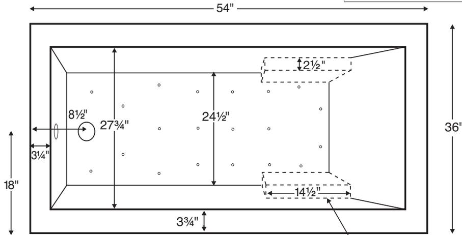
The Sculpted Finish process does not allow enough space for mounting fixtures on the tub deck.
