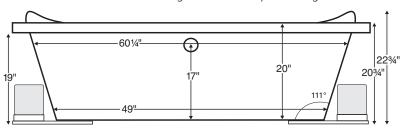
**IMPORTANT:** Air baths and tubs with a pre-leveled foam base or frame system add 2-3" to overall tub height.
