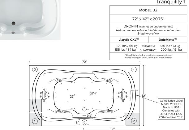
Numbered areas on tub deck represent possible locations to install cleaning systems, faucets and other fixtures. Rear soapdish will be eliminated with Ultra Whirlpool Package. Shown with Air Massage and Ultra Whirlpool Package.
