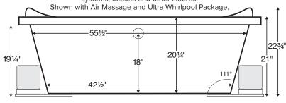
IMPORTANT: Air baths and tubs with a pre-leveled foam base or frame system add 2-3" to overall tub height.
