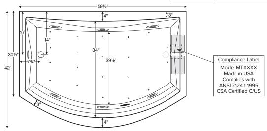
Available with left- or right-hand drain. When ordered with Install Ease frame & skirt package, wall-mount valves are required.
