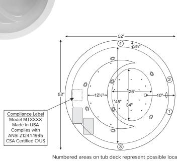
Numbered areas on tub deck represent possible locations to install cleaning systems, faucets and other fixtures. Shown with Air Massage and Ultra Whirlpool Package.
