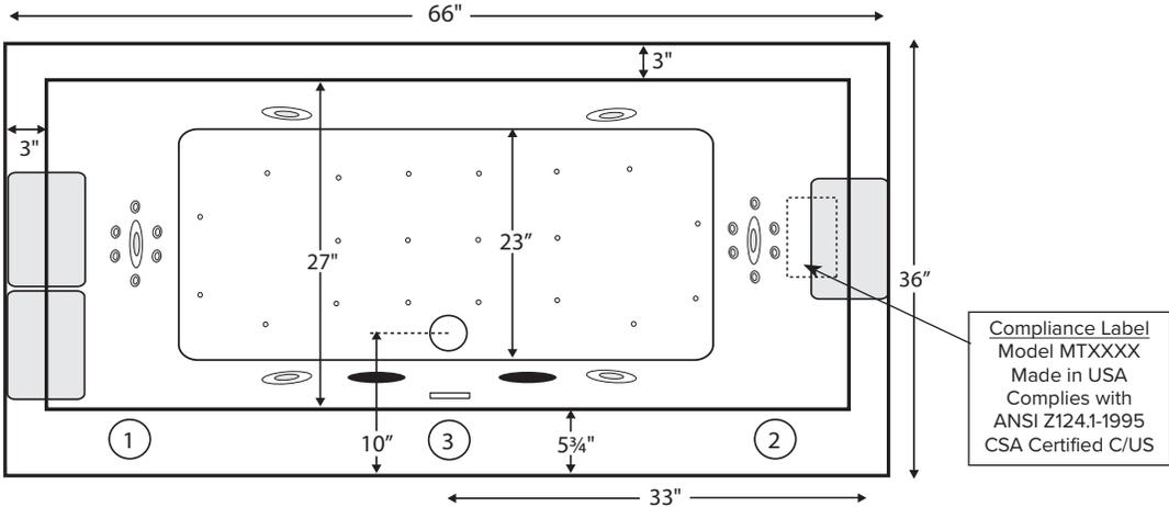
The tub features a round integrated overflow with direct toe tap drain connection directly above rough-in pipe. Numbered areas on tub deck represent possible locations to install cleaning systems, faucets and other fixtures. Shown with Air Massage and Ultra Whirlpool Package.
