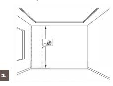
To install the panels on drywall, insert the appropriate anchors and/or locate the studs before drilling. Put the first panel in place and insert the screws, 8 screws per panel, space evenly around the edges.
