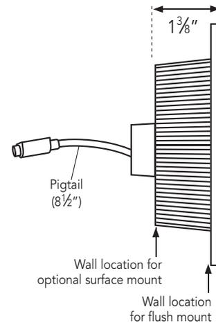
iSteam controls flush mount in the steam/shower enclosure through a 5-1/4" wide x 3-9/16" high hole. iSteam controls can also be surface mounted. They are suitable for use with SteamLinx™ mobile app control.
