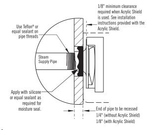
**CAUTION** Consult with supplier of acrylic, fiberglass and other non-heat resistant enclosures for recommended steamhead location. Use Acrylic Shield PN 103938/ 103938SQ. See instructions provided with steam shield. (An acrylic shield is not available for the iSteam steamhead.)
