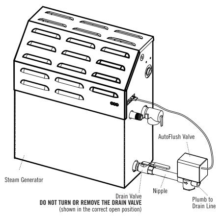
Our exclusive AutoFlush® automatically and electronically drains the system, providing CleanSteam... Every Time® and introduces fresh water.
