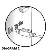
**NOTE:** The connector is keyed with the flat facing up. The control cable is the same at both ends.
