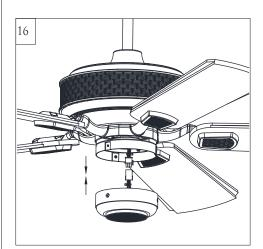
Connect the plug from fan and the plug from switch housing. Make sure the plugs are clasped securely.
