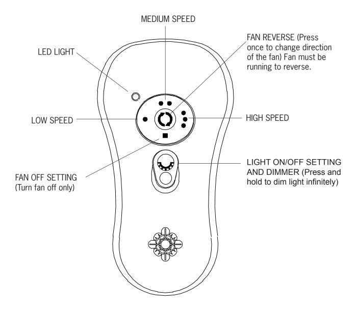
**FAN SPEED**: Depress "1 dot" for low speed, "2 dots" for medium or "3 dots" for high. To turn fan off press square".
