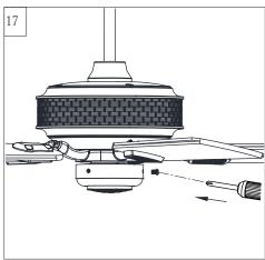
Install switch housing onto top switch housing with the set screws removed in step 15.
