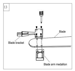
Align the holes of blade bracket, blade and the medallion of blade holder. Install blade bracket with blade by 4 blade screws provided. Tighten screws securely. Repeat this process for remaining blades.
