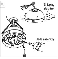
Remove shipping stabilizers from motor assembly.
