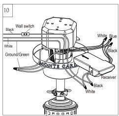
Make wiring connections using wire connectors provided as indicated above. White from fan to White from remote marked N. Black from fan to Black from remote marked L. Blue from fan to Blue from remote marked FOR LIGHT. White from house to White from remote marked AC N. Black from house to Black from remote marked AC L. Connect all green grounded wires to Grounded wire from House. Make sure that no filaments are outside of the wire connectors. Insert the remote receiver into mounting bracket.
