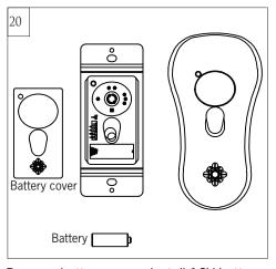
Remove battery cover. Install 12V battery into wall remote. Duracell MN21 / Evereday A23 / GP 23A all 12V. Attach cover of remote by placing over buttons and snap the battery cover in place.
