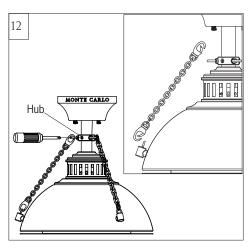
Clip the decorative chains in the rings on top housing and the hub installed on downrod and then pull the hub up until tight and tighten the set screw with downrod on hub.
