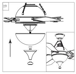
Attached glass onto light fixture and install the silicon washer and hex nut removed in step 17 to hold the glass. Install finial cap and the finial removed in step 17. Hand tighten the finial securely.
