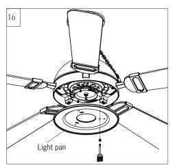
Attach light pan onto the plate on motor, aligning the keyhole slots on the light plate with the preassembled screws on the plate. Twist clockwise till lock. Reinstall the screw removed in step 15. Tighten all screws securely.
