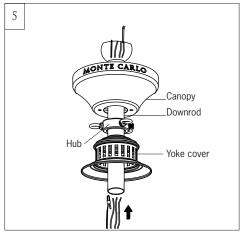
Place downrod over canopy, hub and yoke cover. Thread lead wires and safety cable from motor assembly through downrod.
