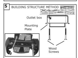
Secure mounting plate directly to a joist from the buliding structure via the two knock out holes on the outlet box. Use only the appropriate wood screws and washers included with your fan. Caution: Wood screws must go through into the building joist.
