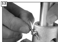
Insert downrod into motor yoke.
