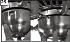
Align the reverse switch preassembled on switch housing with the long slot on switch housing cover as shown and then install the switch housing using the 3 screws previously removed.
