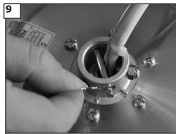
Remove the keeper pin and cross pin.
