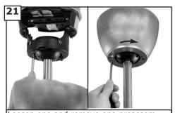
Loosen one and remove one preassembled screw from mounting bracket. Save screw. Lift canopy up, aligning its keyhole slot with the preassembled screw on mounting bracket and twist clockwise to lock in place. Re-install the removed screw and tighten all screws securely.
