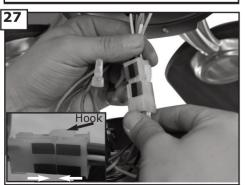
Connect plug from fan to plug from switch housing. Make sure the plugs are hooked together.
