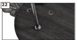
Install 3 screws and washers per blade and tighten securely. Repeat for all 5 blades (Blades sold separately).
