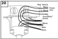
Make wiring connections as indicated above. Connect black and blue wire from fan to Black or (Hot) wire from house. Connect White wire from Fan to White (Neutral) wire from house. Connect Ground leads from mounting bracket and downrod to Ground lead from house. Refer to Safety Tips section of manual.
