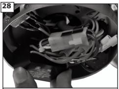
Attach capacitor onto switch housing by preadhered double-sided foam tap as shown.
