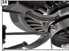
Remove the 3 screws on the switch housing cover and save.
