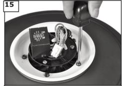
Remove the shipping stabilizer by removing the set screws and discarding.
