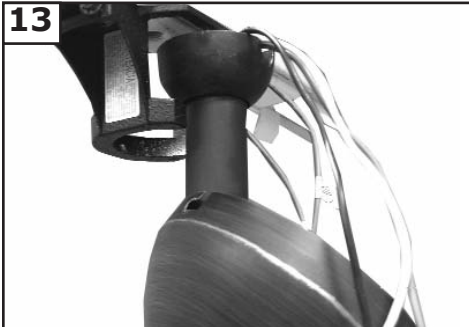
13 Hang assembled fan from the mounting bracket installed to ceiling in previous step. Make sure the fan is hanging straight. Rotate fan until the tab on the Mounting bracket engages the slot on the Downrod Ball. This must be done to prevent the fan body from rotating when the blades are in motion.
