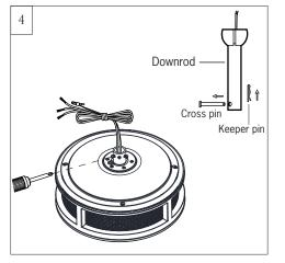
Partially loosen downrod set screws from yoke at top of motor assembly. Remove preassembled cross pin and keeper pin from downrod.
