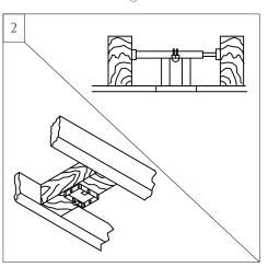
Before installing this fan make sure the outlet box is properly installed to the house structure. To reduce the risk of fire, electric shock, or personal injury, mount to outlet box or supporting system acceptable for fan support. (Mounting must support at least 35 lbs.)
