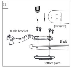
Align the holes of blade bracket, blade and the bottom plate of blade bracket. Install blade bracket with blade by 4 blade screws provided. Tighten screws securely. Repeat this process for remaining blades. Note: Make sure the side with a label "This side up" is installed upward.
