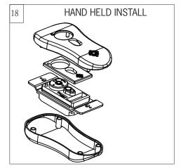
Place battery cover over battery compartment and buttons. Place remote over 2 pins on front cover. Attach cover of remote by placing over 4 pins and snapping into place.
