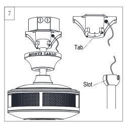
Install ball end of downrod into mounting bracket opening. Align (engage) slot on ball with tab on mounting bracket. Warning: Failure to align slot on ball with tab may result in serious injury. **Important**: If using the angle mount, make sure open end of mounting bracket is installed facing the higher point of the ceiling and make sure the ceiling angle is not steeper than 30°.
