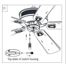
Remove 3 set screws from top plate. Keep screws.
