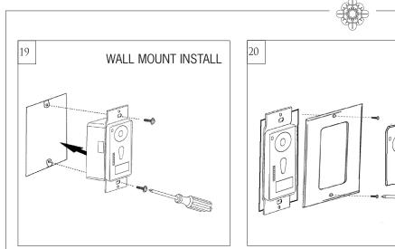
Install wall control unit to outlet box using machine screws provided.
