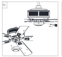
Attach switch housing onto top plate, aligning the holes and reinstall the 3 set screws removed in step 15 and tighten all screws securely.
