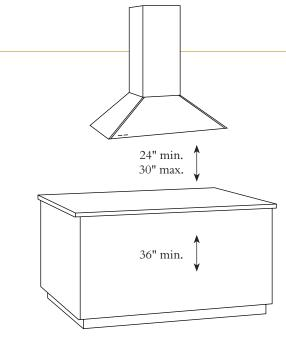
The exact installation height is determined by the ceiling height and duct cover trim strips provided with the hood. For optimum performance, the hood must be installed 24" min. and 30" max. above the cooking surface.
