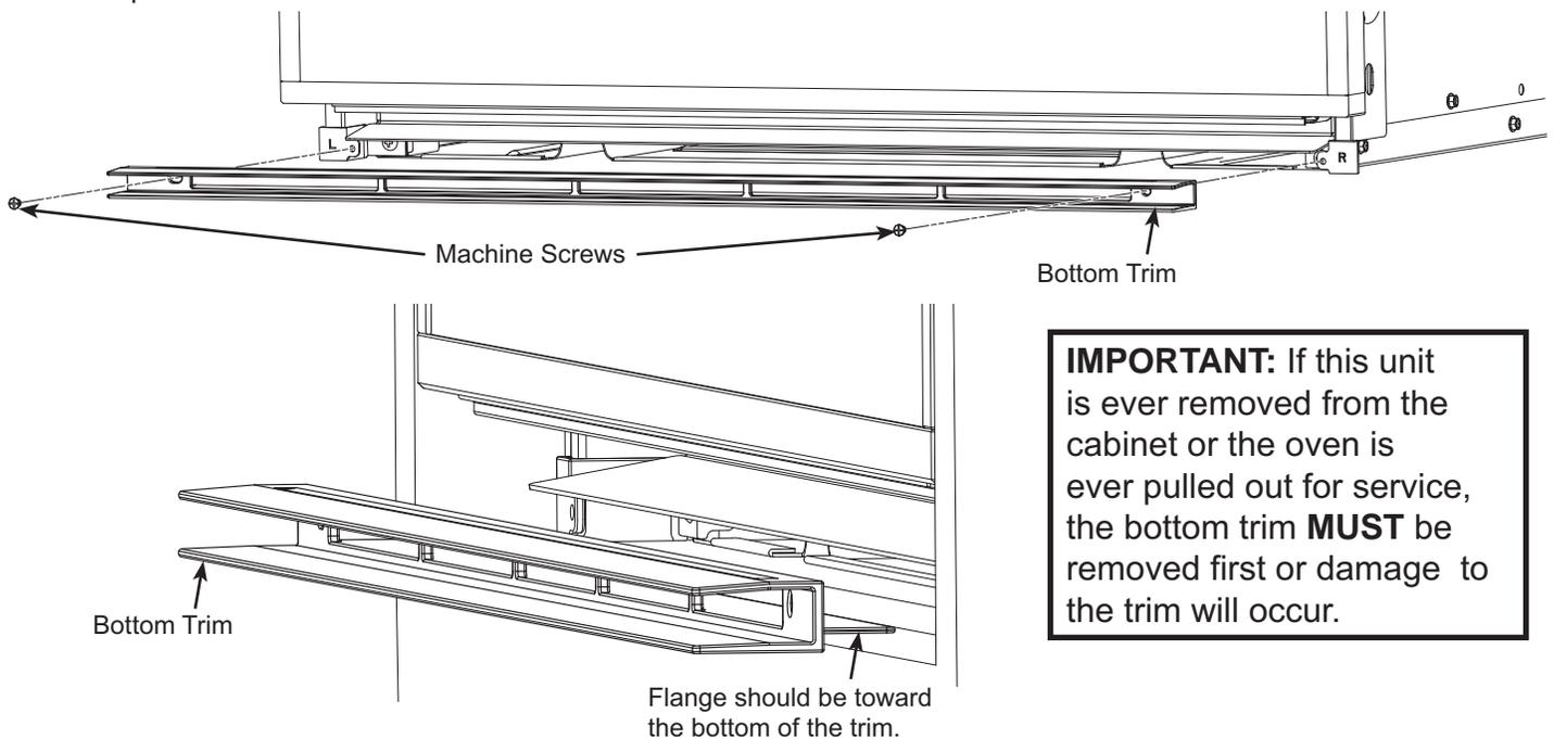
**IMPORTANT:** If this unit is ever removed from the cabinet or the oven is ever pulled out for service, the bottom trim **MUST** be removed first or damage to the trim will occur.
