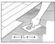
NOTE: Never work on top of the flooring when installing. If you must work on top of the newly laid flooring, use a kneeling board.
