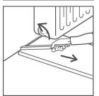
If it is difficult to tilt the planks (e.g. under radiators), use a pull bar installation tool to pull the planks together.
