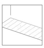
Begin in the left corner of the room. Install underlayment, if needed. If you choose to use underlayment install it simultaneously with the floor installation. We recommend Mohawk ActiveSound Underlayment which helps ensure joint integrity, reduces sound, helps prevent indentation, and insulates and helps level the subfloor. SolidTech products with pad attached cannot be installed over separate underlayment
