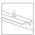
Then slide the third plank together horizontally. Slightly lift the plank to be installed by holding your hand underneath. Push the short side joint down gently with your thumb moving from the inner corner towards the outside until you hear a "click". Ensure the short side ends are closed by knocking gently on the short side click connection with the palm of your hand or tapping block
