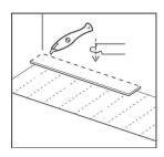
Begin in the left corner of the room. Start the first row with a whole plank. Cut off the long side tongue (end and edge) for the first panel. Position the cut edges adjacent to the wall.
