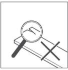
Visually inspect all planks before and throughout installation in optimal lighting. Defective planks should be discarded or, when possible, used as cut pieces to start or finish rows after removing the defective portion of the plank.
