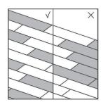
During installation, blend the planks so that there are not too many identical, lighter or darker panels adjacent to one another. For optimal results, it is best to fit the panels in the direction of the longest wall and parallel to the light source in the room. Ensure that the end joints of the panels in two successive rows are never in line, they should be staggered by at least 8 inches.
