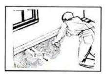
Use Uniclic Tapping Block if necessary to fit planks snug together at side and butt ends. Clean any adhesive off the surface before it cures using clean terry cloth towels and mineral spirits.
