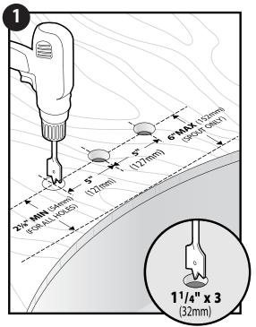
1) Drill holes for the valves and spout 5" minimum on center. Position the spout hole so that spout delivers the water to the desired place in the tub.
