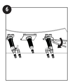
6) Secure valves & shank, tighten lower nut **firmly** using pliers.
