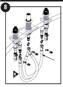
8) Secure the hose assembly with quick connect clips (M). For 5" – 8" centers between the valve and spout shank, loop the hose (K) as shown. For 9" – 12" centers, do not loop.
