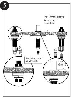
5) When properly assembled, top nuts (D) are below notch on each valve. On center shank, leave 1/8" of threads above deck.
