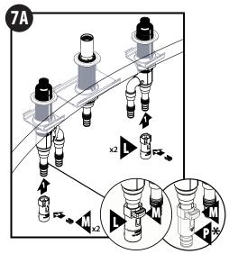
7A) For CPVC or Cold expansion connections, attach the adapters (L or P) onto the straight inlet over the "O"-rings. Insert (M) into connector as shown.
