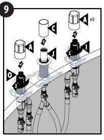
9) Place protective tube (C) over center shank assembly (J) and protective caps (A) over valves (I & O).
