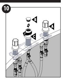
10) Secure protective tube (C) with test plug (B).
