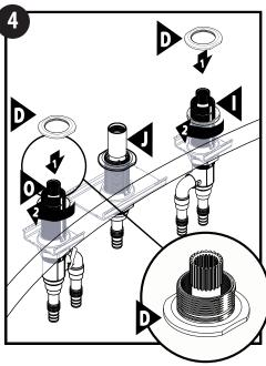
4) Thread top mounting nuts (D) to slightly below notch on each valve (I & O) and spout shank (J).
