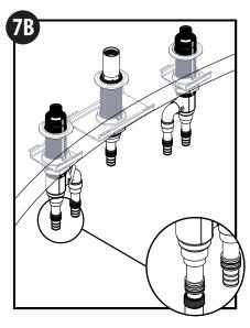
7B) For PEX connections slide tubing onto the straight inlet tubes up to the "O"-ring and crimp the banding ring with a crimping tool.
