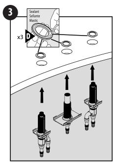
3) From the underside of the deck, insert completed assemblies. Position both valve assemblies so the shorter legs (outlets) face towards the center shank assembly. Add bead of sealant on bottom of top nuts.
