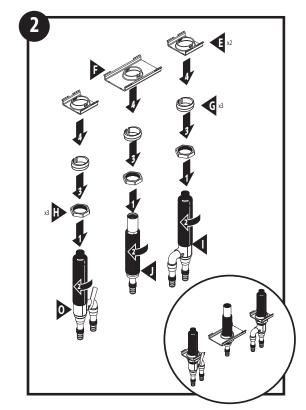
2) Assemble nut (H), tapered bushing (G) and valve bracket (E) onto valve assemblies (I & O). Assemble Nut (H), tapered bushing (G) and shank bracket (F) onto shank assembly (J).
