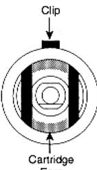
time of rough-in and trim out. If the retainer clip is not properly installed, water pressure could force the cartridge out of the casting. Personal injury or water damage to the premises could result.
