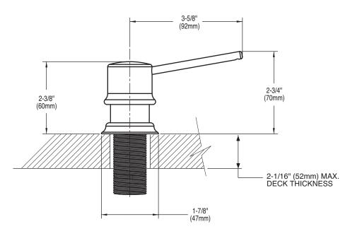
**NOTE:** DESIGNED TO BE INSTALLED THROUGH 1 HOLE 1-1/8th MIN. - 1-1/2 MAX . DIAMETER
