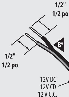
Measure and cut a Dual Strand 18 ga. Wire (B)\* to the length. Strip about 1/2" of the insulation off both ends of each strand of 18 ga. wire.
