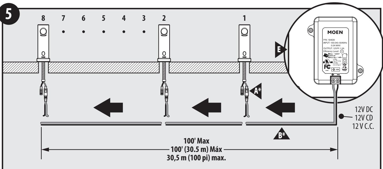
Run the Dual Strand18 ga. Wire (B\*) from the Transformer (E) to each Fixtures' Power Cable (A)\*.
