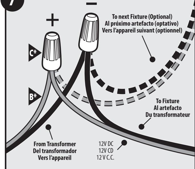
Using Wire Nuts (C)\*, connect each strand of the Dual 18 ga. Wire (B)\* to one of the two output lead wires of the transformer, as shown. Ensure that the strand of the 18 ga. wire extension that is connected to the positive (+) output lead wire of the transformer is connected to the gray lead on the fixture's power cable. **Optional:** Using wire nuts, include the next leg of power in the connection). **Note:** For wire drywall exit location, see schematic below.
