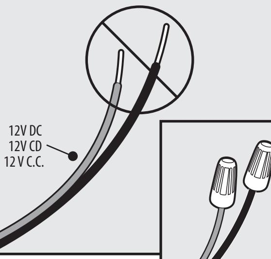
Properly terminate all connections. There should be no open leads exposed.
