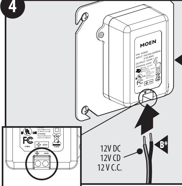
Strip about 1/4" of the insulation off of the ends of Dual Strand 18 ga. Wire (B)\*.
