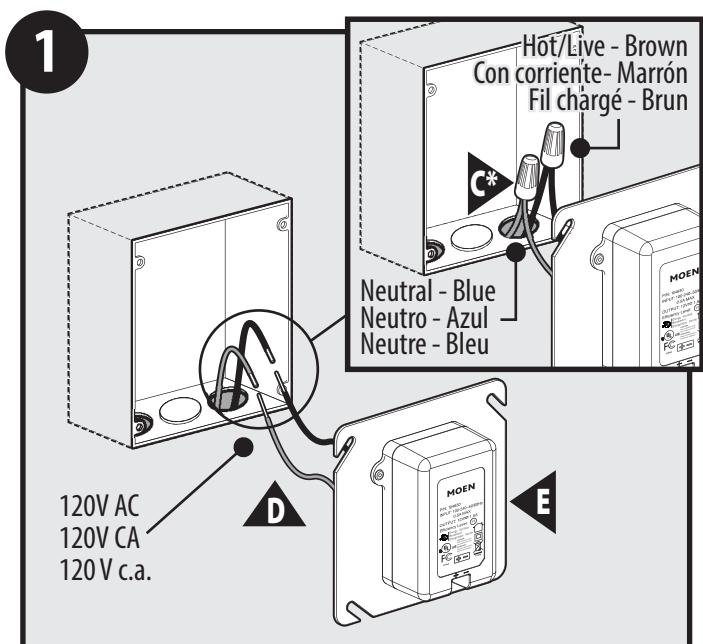
**Note:** Ensure breaker is turned off prior to connection. Connect Transformer Input Lead Wire (D) to junction box with Electrical Wire Nuts (C\*). **Caution:** A disconnect device that is in close proximity shall be provided as part of the building installation.
