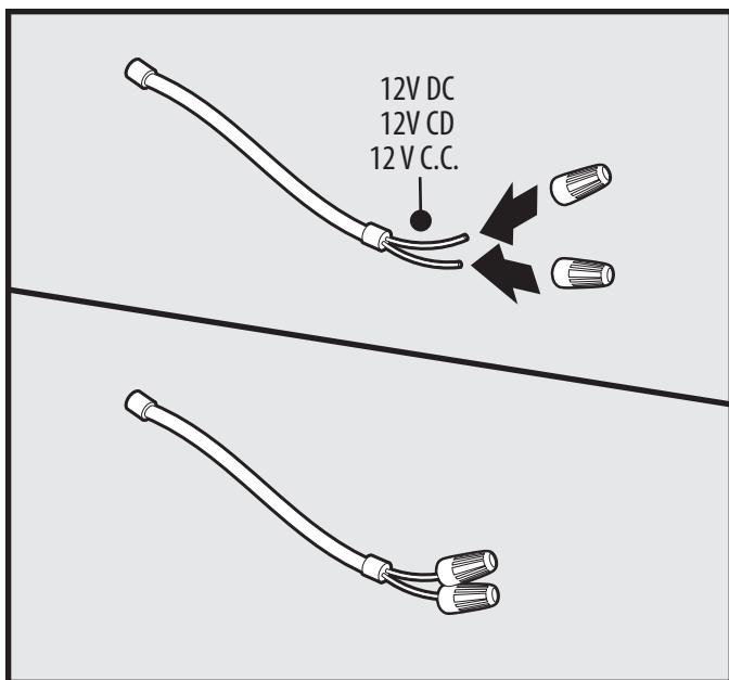
**⚠ Warning:** Do not touch bare ends of transformer output lead wires together when transformer input lead is plugged into electrical wall outlet; avoid contact by using electrical wire nuts as shown during installation.
