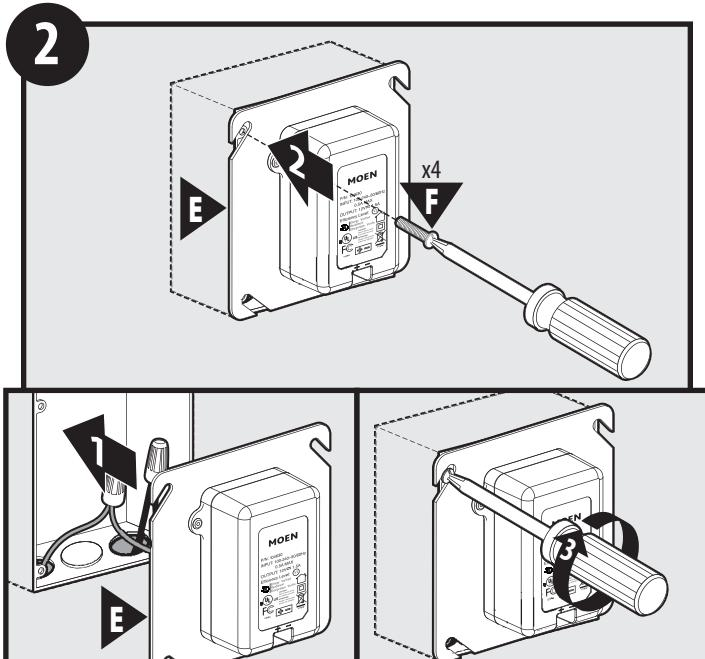
1. Hold Transformer (E) up to junction box, ensuring wires are not pinched.
