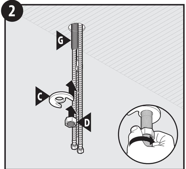
Slide mounting bracket (C) up onto shank of faucet body (G) under sink and secure with mounting nut (D).
