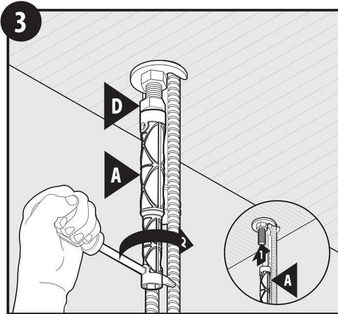
(1) Tighten mounting nut (D) with mounting tool (A). (2) Use screwdriver through hole in mounting tool (A) to tighten firmly.
