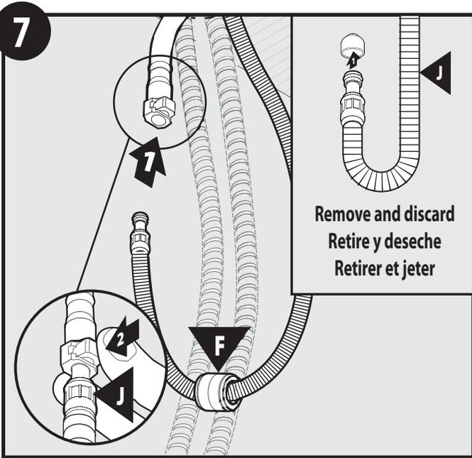
Remove protective cap (see inset). Attach wand hose (J) into quick connect on outlet hose (I). Push into connector and push clip until click is heard. Pull down to check that connection is secure.
