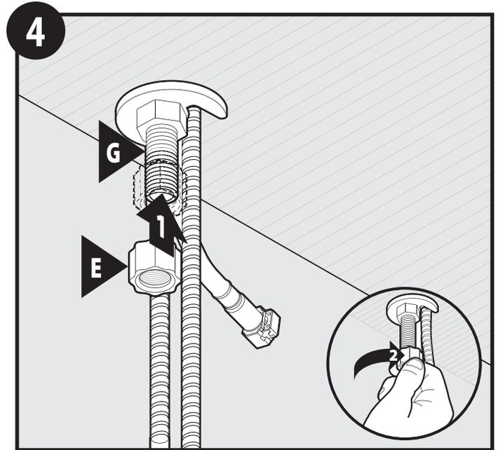
Secure hose guide (E). Thread hose guide (E) onto faucet body (G) until secure.
