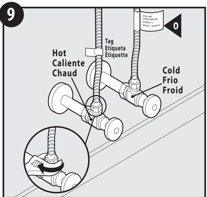
Connect water supply lines, and secure with wrench. Insert ID label (O) to hose as shown.
