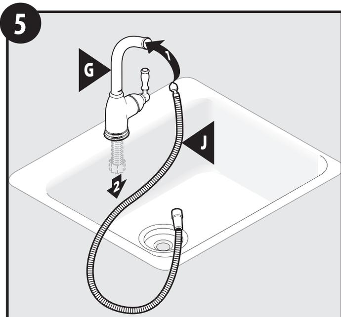
Insert small end of wand hose (J) into spout and feed through faucet body (G).
