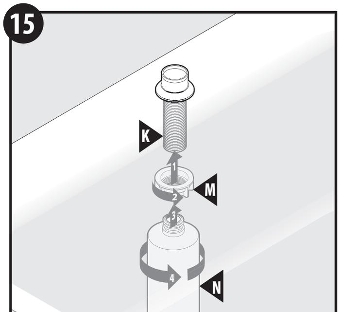
Thread mounting nut (M) to soap dispenser underneath the deck. Thread bottle (N) to bottom of soap dispenser until secure.
