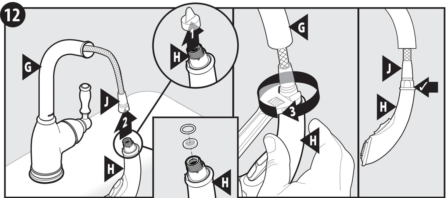
Remove and discard protective cap from wand (H). Ensure that the screen and rubber washer are in the inlet of the wand. (Verify that the flat washer is in the hose fitting.) Thread hose on to wand assembly. Insert wand into spout until seated.
