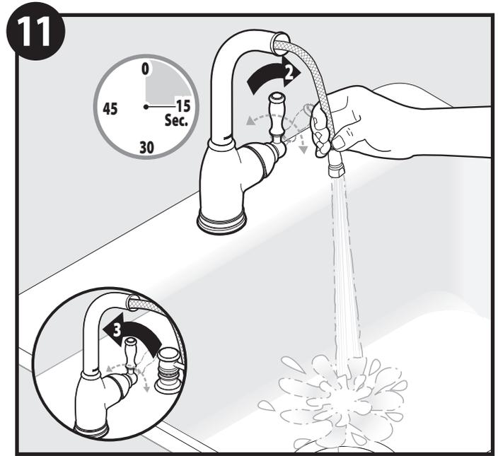
To flush debris from the plumbing system: Hold the hose, run hot and cold water for 15 seconds as shown.
