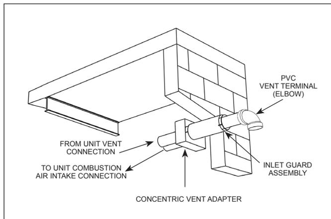
Figure 11.2 - Vertical Concentric Vent Kit
